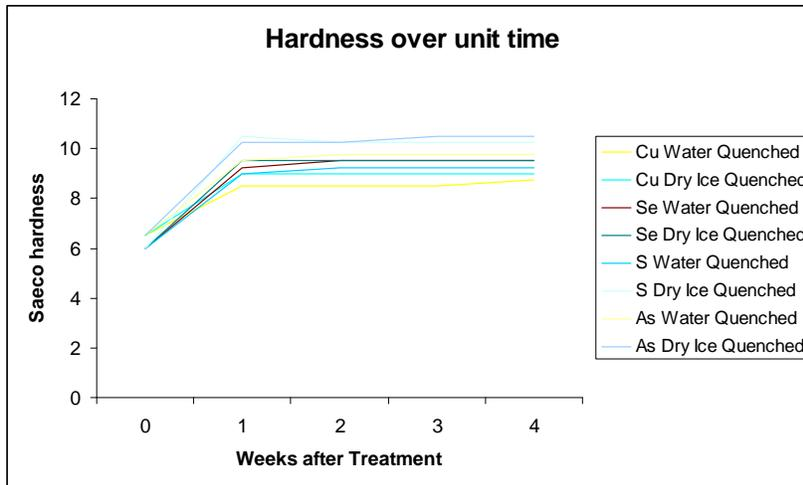
As expected, all the grain refiners worked in the same way and with only mild variations in final strength regardless of the quenching method used. All showed similar patterns of the most significant gains being present by the end of one week with slight continued strengthening over the
