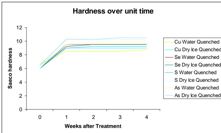
As expected, all the grain refiners worked in the same way and with only mild variations in final strength regardless of the quenching method used. All showed similar patterns of the most significant gains being present by the end of one week with slight continued strengthening over the next 3. This is not atypical of other Hall-Petch strengthening results as dislocation will continue at a slow pace after hardening.
