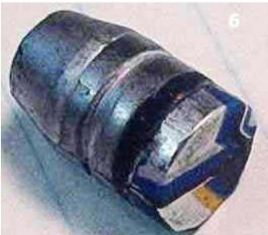
I used Freechec's on the bullets and ran them to 1500 fps with no leading problems. I shared this with the manufacturer and they redesigned the bullet with a single large flat lube groove. That solved the leading problem, and we no longer used the Freechec on them. But the Freechec allowed a marginally lubed bullet to run at much higher velocity and pressure than normal. And do it well.
