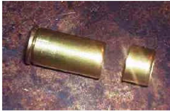
Once the cartridge is cut I expand the neck with a tapered plug to allow the pilot of the case trimmer to enter the cartridge. An old .50 caliber machine gun bullet works just fine.
