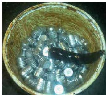
When designing this bullet we made the grease grooves fairly small and lubing that way gives some leading as velocities get over 800/850 fps.
