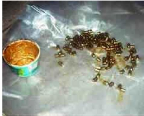
Put the lid on the container, hold on tight and shake it around and up and down and around and around ... hey! A rock 'n roll song! Do that for a few minutes until all the bullets have a good covering of lube.
