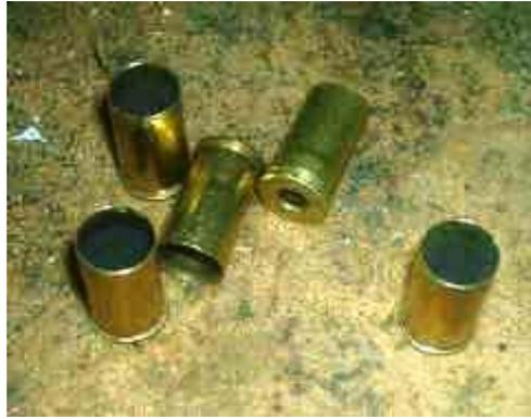
When the case is trimmed to length then I chamfer and de-burr. The cartridges are now ready for final neck expansion to allow bullet seating. They can then be primed and loaded.
