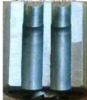
Cut-Away cylinder Note the step where it goes from cartridge diameter to bullet diameter
