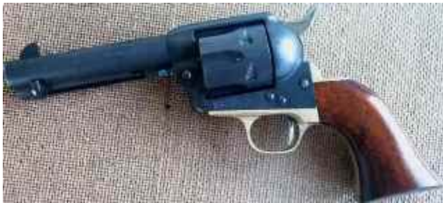
backstrap and trigger guard are of brass instead of steel.
