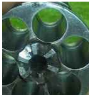
Looking through a normal chamber you can see the "step"
