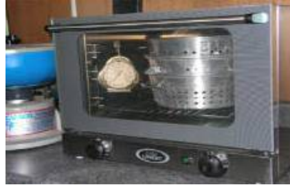
Convection oven, a thermometer and the spaghetti pans. Any bullets too long for bottom or middle pan are done in top pan.
