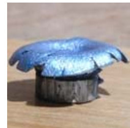
Stick-on WW, 45 ACP 200 gr. HP @ 800-850 fps fired into water.
