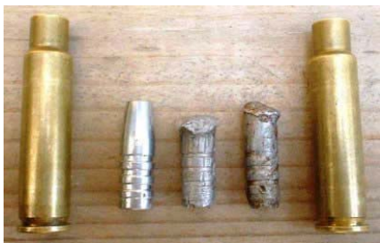
Recovered bullets -- fired .338 GEF cases, the MM 235 as-cast (left), recovered first shot (center), and second shot (right)
