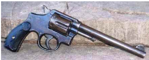
The Model 1899, aka .38 Military & Police First Model. The first .38 Special. Note the lack of a lug on the bottom of the barrel.
