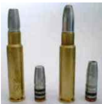
The .338 GEF, the 235 grain Mountain Molds GC-FP (left) and the Lyman 33889 hollow-point (right).
