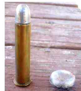
The unfired bullet weighs 393 gr. The recovered bullet weighed 385.6 gr.
