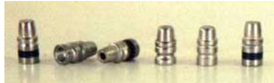
The family of .38 Keith SWC's: the Lyman 358429 SWC, the Hollow-Base 358431, the Hollow Point 358439, the 358477 (150 grain version), the 358477 (158 grain version), followed by another 358429.
