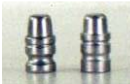
A close up showing the differences between the 150 grain version of the 358477 (left) and the 158 grains version of 348477 (right).
