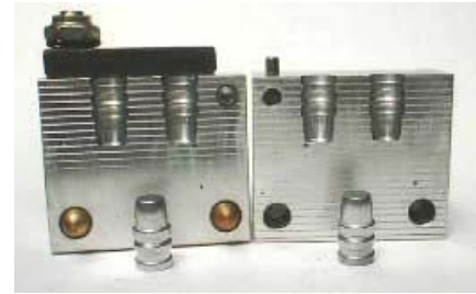
.32 caliber Keith-style SWC for the .32 H&R Magnum made by Mountain Molds.
