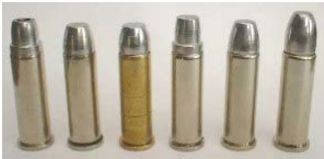
Some of the bullets that worked well in the .357 Marlin when loaded into .38 Special cases: the Lyman 358439, the Lee 358-158-RF, the Lyman 358665, the Lyman 358429, the LBT 200 LFN and the Lyman 35875 200 grain RNFP.
