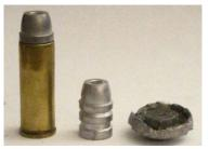
1102 fps. According to the pressure data in the Accurate Arms loading manual, this combination should generate roughly 19,000 CUP. This would make an excellent hunting load.
