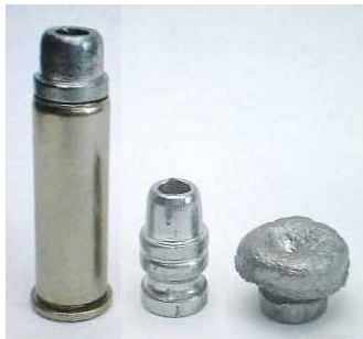
Loaded .38 Special round with a 358477 HP cast to a BHN of about 8, and a recovered bullet after being fired into water at about 1000 fps.
