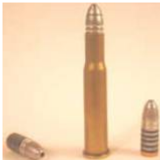
The .30-30 Winchester loaded with the 157 grain Lyman 311466 HP. Expansion of this bullet at 1800 fps is violent.
