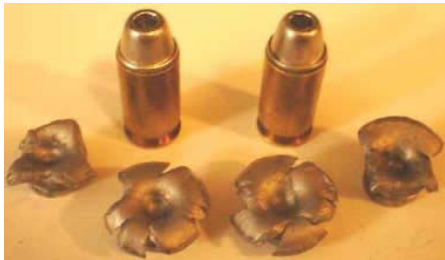
Lyman 452460 HP and expanded bullets (fragmentation due to alloy used in test bullets)
