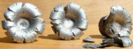
Lyman 452374 Devastator fired straight down into 3 feet of water with 6.5 Gr unique at 850 fps, alloy is clip-on WW plus 3% added tin. Even at this modest velocity some of the bullets noses broke off with the 2-3% antimony alloy.
