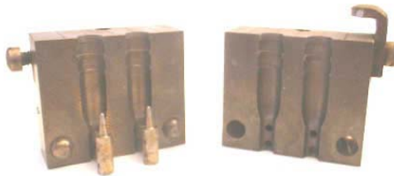
Repaired Cramer #41B mould.
