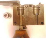
Early Ideal HP moulds had no "keepers" to hold the HP pin in (e.g. the old Ideal 25727 mould shown (top)). After 1940, Lyman HP moulds had keeper pins to hold the HP pin in place (e.g. the 454424 HP mould shown (bottom)), and after about 1990 they used a snap-ring to hold the pin in place (e.g. the 429244 HP mould shown (center)).
