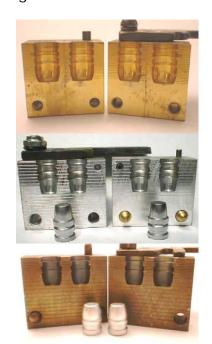
Bullet moulds can be made out of many materials. Popular materials include brass (Applegate 45 315 WFN mould, top), aluminum (Mountain Molds .40 caliber 200 grain Keith-style SWC, middle), and various ferrous alloys (RCBS 40 180 Cowboy mould, bottom).
