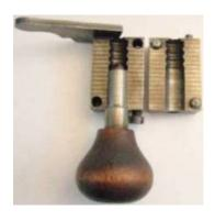
Classic wadcutter bullet moulds: the Ideal 358395 hollow-based wadcutter.
