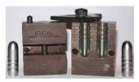
An example of an Ideal 2-cavity mould (308291).
