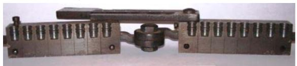
Tools to gladden a sixgunners heart! H&G gang moulds, cut to Elmer Keith's specs for the Keith SWC's
