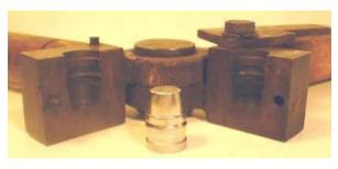
A copy of the Ideal 452423, made by Yankee Specialty Co. with integral handles (Yankee Specialty also made a few moulds with interchangeable blocks). This Depression-era mould is made from bronze, not iron.
