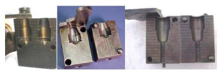
Examples of the Harvey Prot-X Bore cast bullet designs (e.g. the .38 and .45 Harvey moulds shown). Some of the Harvey designs were even available in HP form (e.g. the .44 HP mould shown).
