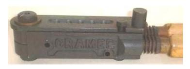
A Cramer 5 cavity .38 wadcutter mould.
