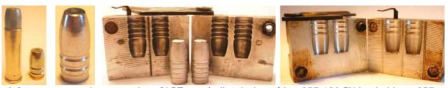
A few representative examples of LBT cast bullet designs (the .357 180 FN loaded into .357 Magnum, the LBT .357 200 grain LFN-GC, the LBT .417 305 grain LFN, the LBT .432 320 grain WLN.
