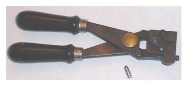
Picture of a Modern-Bond F-257-730 mould (a .25 caliber 86 grain GC-RN), showing the unique black lacquered handles of the Modern-Bond moulds.
