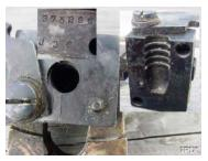
An example of a 2-part bullet (Ideal 375296). The small mushroom-shaped tip would be cast out of a soft alloy (like pure lead), then that piece would be inserted into the regular cavity of the bullet mould and the remainder of the bullet would be cast of somewhat harder alloy.
