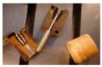
Mould blocks after HP channel has been drilled out, and the roughed out HP pin and knob.
