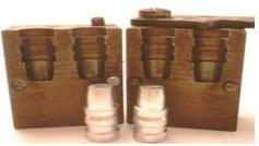
Early revolver bullet designs did not include a dedicated crimp groove (e.g. the Ideal 360271 and 360345 target bullets shown at left). Elmer Keith integrated a beveled crimp groove into the Ideal/Lyman 358429 (right) and most revolver bullets designed since then have followed suit.
