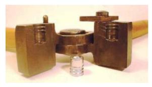
Note the lack of alignment pins and the handcut vent lines.
