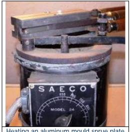
Heating an aluminum mould sprue plate down
