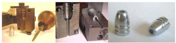
The first HP moulds suitable for use in handguns. These bullets were designed as "express bullets" for use in rifles, but also could be fired in revolvers (all were listed in the Ideal Handbook #9, circa 1897); the Ideal 31133 HP for the .32-20; Ideal 40090 HP for the .38-40, and the Ideal 42499 HP for the .44-40.
