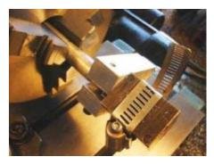
452460 mould clamped onto mandrel and held in place with dog.
