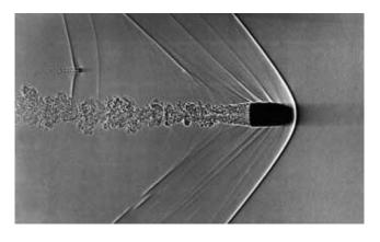
A shadowgraph of a supersonic bullet in flight. Note the bow wave -- how the ogive of the bullet interacts with this bow wave can have a significant impact on the stability of the bullet's flight. Note also the smaller pressure waves emanating from the grease grooves. Photo courtesy of: http://www.efluids.com/ efluids/gallery/gallery\_pages/bullet shadowgraph.jsp
