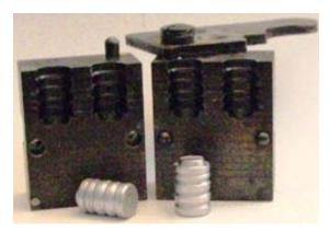
An example of a bevel-based wadcutter mould (Lyman 358091).
