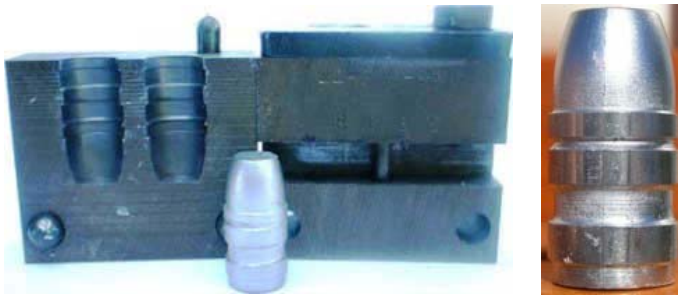
RCBS 44 300 Gr. SWC GC Mould and Bullet.
