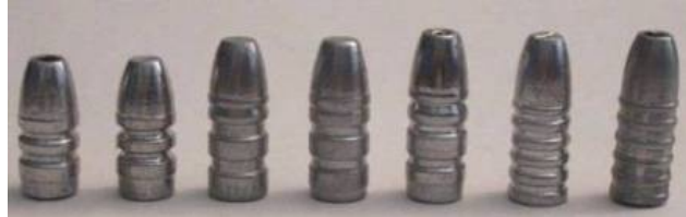
Cast bullets used in this loading project; (l-r) Lyman 257420 HP, 257420 solid, Ideal 257283, H&G #54, Ideal 257312 HP, Ideal 25720, and Ideal 25727 HP.
