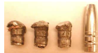
The Lyman 33889 HP, as-cast, and recovered after being expansion tested at 1600 fps.
