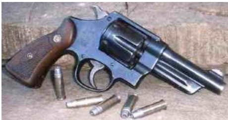
Elmer Keith used the N-frame .38 Special to develop the .38/.44 loads that ultimately led to the .357 Magnum. This is the .38 Heavy Duty (circa 1950).
