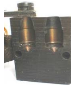
The Lyman 357500 Harvey Pro-Tex Bore SWC mould (the slot at the base of the bullet is where the zinc washer fits into the mould prior to pouring the molten alloy into the cavity; the conical rivet below that is what holds the washer in place).
