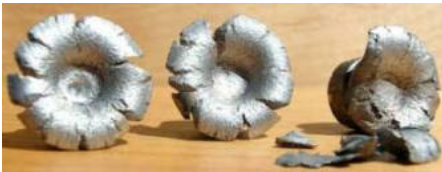
Lyman 452374 Devastator fired straight down into 3 feet of water with 6.5 Gr unique at 850 fps, alloy is clip-on WW plus 3% added tin. Even at this modest velocity some of the bullets noses broke off with the 2-3% antimony alloy.
