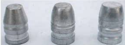
Bullets that were found to shoot well out of the S&W 696 .44 Special (l-r: the Saeco 200 grain TC, the Cramer 8A 220 grain RNFP and the LBT 237 grain WFN).
