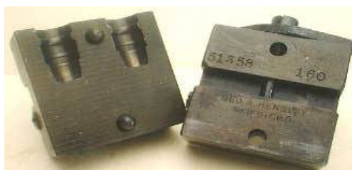
George Hensley #51 -- the "Sharpe solid" used in the development of the .357 Magnum cartridge (this mould pre-dates Hensley's 1937 partnership with James Gibbs, making it contemporary with the introduction of the .357 Magnum).
