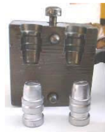
The 160 grain Hensley # 51 ("Sharpe solid"), the original .357 Magnum bullet.
