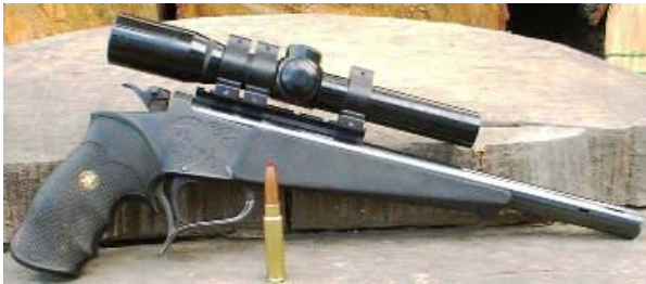
The .338 GEF Contender (12" barrel) and a round loaded with the Nosler 200 grain Ballistic Tip.
