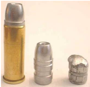
44 Mag w/RCBS 300 Gr HPGC & expanded bullet (recovered after being shot through a gallon jug, into dry newsprint and both are tough on a bullet, this HP held up very well).
