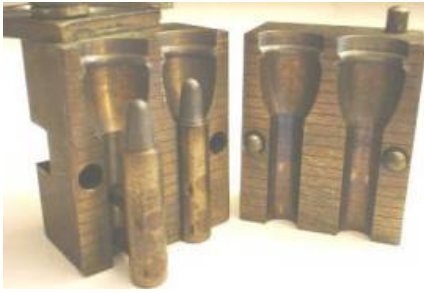
The Cramer-style HP conversion on the Ideal 452374 2-cavity mould.
