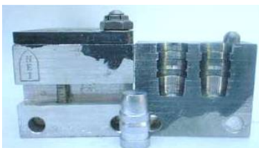
The NEI #256 (.44 SWC, 270 grains WW alloy).
