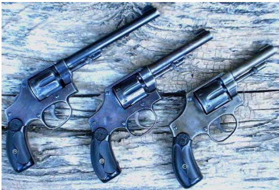
The I-frame .32 S&W Long (Model 1903) was available with 3 1/4", 4 1/4" and 6" barrels.
