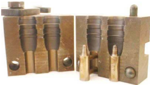
RCBS 44 Caliber 300 gr. SWC GC Converted to Cramer style hollow point By Erik Ohlen - Hollow Point Bullet Mold Service
