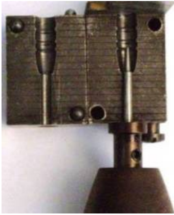
The Ideal 257312 mould after Erik Ohlen converted it to make HP bullets.
