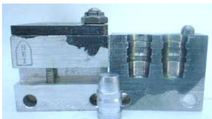
The NEI #256 (.44 SWC, 270 grains WW alloy).
