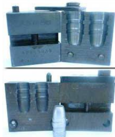
The RCBS 44 300 GC-SWC, and the Lyman 429650 GC-SWC (310 grains WW alloy).
