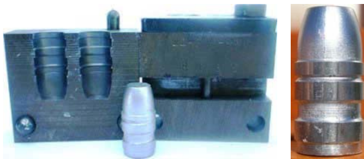
RCBS 44 300 Gr. SWC GC Mould and Bullet.
