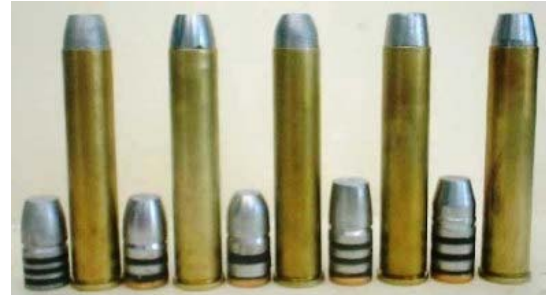
Some of the bullets tested in the 444 Marlin. (l-r: LBT 430-300-LFN, 280 grain Lyman 429640, Saeco 300 grain RNFP, LBT 430-350-WLN, and NEI 429-330-GC).
