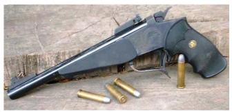
10" T/C Contender re-chambered from 10mm to 40-50 Sharps Straight, loaded with the Lyman #403169.
