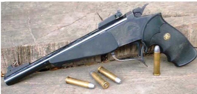
10" T/C Contender re-chambered from 10mm to .40-50 Sharps Straight, loaded with the Lyman #403169.
