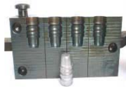
The Lyman 358156 GC-SWC; probably the most popular cast bullet ever for the .357 Magnum
