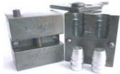
The Ideal 311316, the first SWC suitable for handguns to have a beveled crimp groove.
