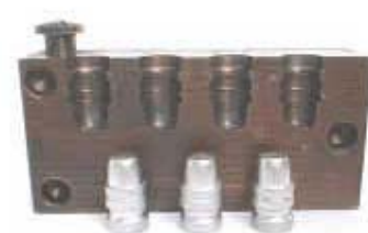
The 150 grain Lyman 358477 SWC; a fine bullet for both .38 Special and .357 Magnum.
