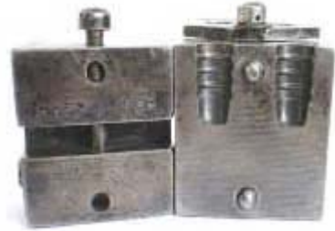
The H&G # 48 158 grain SWC (no beveled crimping groove)
