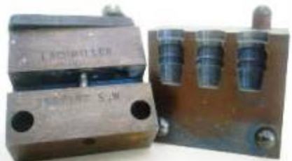
Lachmiller 3-cavity 358 158 SWC mould.
