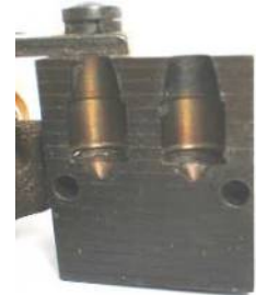
The Lyman 357500 Harvey Pro-Tex Bore SWC mould (the slot at the base of the bullet is where the zinc washer fits into the mould prior to pouring the molten alloy into the cavity; the conical rivet below that is what holds the washer in place).
