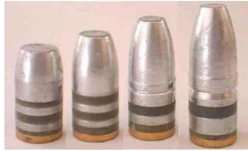
The cast bullets used in the .35 Remington- the LBT 358-180-WFN, the LBT 358-200-LFN, the RCBS 35-200-FP, and the Saeco #352 (245 grain FPGC).
