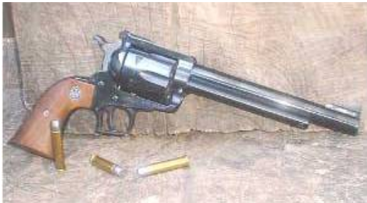
The Ruger .357 Maximum Super Blackhawk revolver, built on a stretched Super Blackhawk frame. This revolver was available in 7 1/2" and 10 1/2" barrel lengths.
