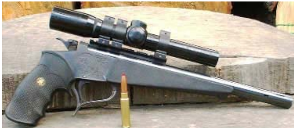
The .338 GEF Contender (12" barrel) and a round loaded with the Nosler 200 grain Ballistic Tip.
