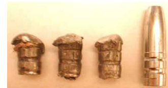
The Lyman 33889 HP, as-cast, and recovered after expansion tested at 1600 fps.
