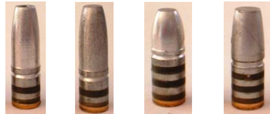
The cast bullets used in these tests: (l-r) Lyman 33889 HP, Lyman 33889 GC-FP, RCBS 200 grain GC-FP, and the Mountain Molds 235 grain GC-FP.
