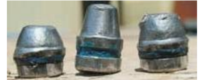
SAECO # 068 200 gr. 45 Caliber SWCBB 5 BHN fired at 800 fps into 3 feet of water and hit the bottom of the plastic drum
