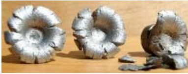
Lyman Devastator HP 202 Gr. 45 caliber fired into 3 feet of water at 800 fps - 11 BHN
