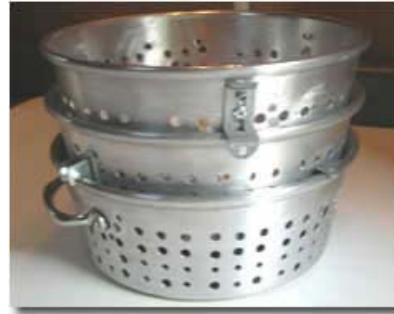
Aluminum Spaghetti pans with holes enlarged for better water flow. Each pan holds nearly 300 35 caliber bullets.
