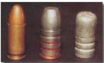
Photo 1 L-R - A standard gmmP cartridge alongside a pristine 420gr gas-checked cast bullet and the one recovered from the buffalo. This impressive performance disappointed the author.
